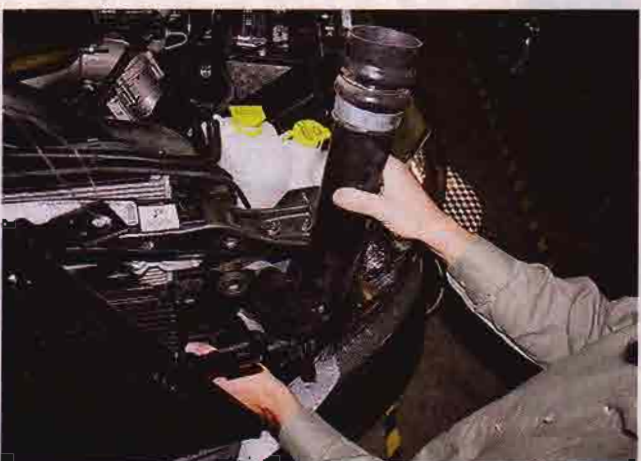
10. Install 3 1/2-inch hump coupler to manifold with clamps provided.
