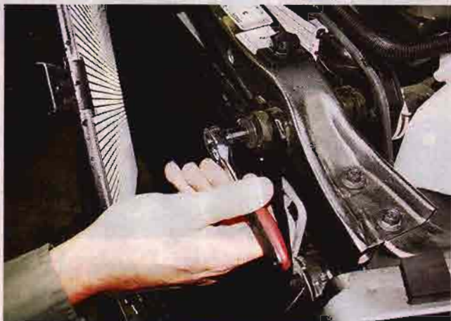
5. Using a 10mm socket or wrench, remove the two top intercooler attachment bolts connected to upper radiator support.
