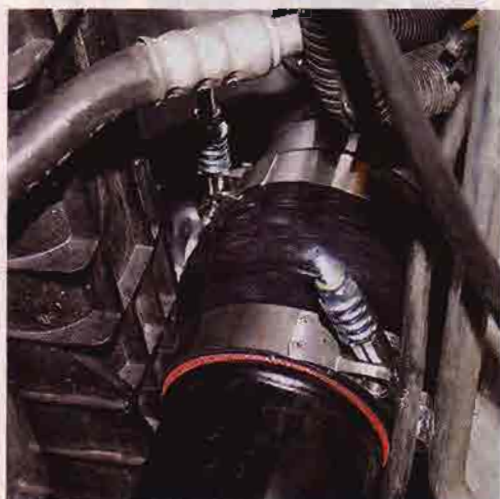
17. Reattach A/C line protector. Reinstall intake/stock air box and reconnect battery. Your installation is now complete. Check all screws and clamps periodically. Retighten if necessary.
