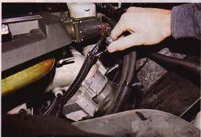
9. With a 7/16-inch-deep socket, loosen clamp on manifold. Push down on intercooler tube and disconnect from manifold.
