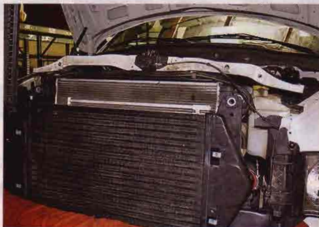
8. Remove the upper radiator support and set it aside on the top of the fan shroud. Loosen clamps on intercooler tubes using 7/16-inch-deep socket. Now remove stock intercooler and factory couplers/clamps out of the vehicle.
