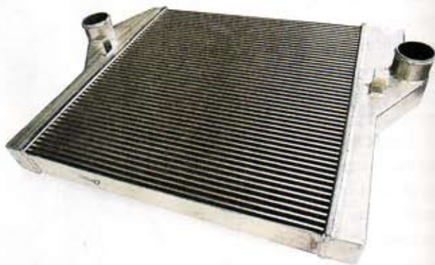
9. You might not realize how much stress is being exerted on an intercooler, but on a big core like this, at 30 psi there's more than a ton of force trying to push the end tanks in opposite directions. Combine that with exposure to the elements, (not to mention the occasional hailstorm, gravel truck or road alligator), and you'll understand that material quality and workmanship are extremely important.
