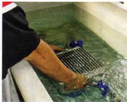
8. Ideally, intercooler cores should be 100-percent leak-free, but very small pinholes (0.05 cfm or less) are considered within spec, since the hose clamp connections at the tanks typically leak more than that.
