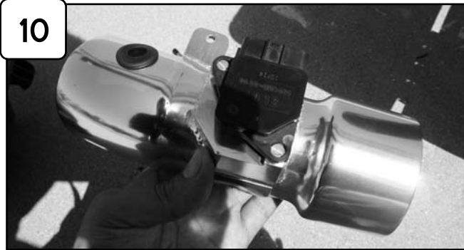
Install grommet to tube. With M4 screws provided secure MAF sensor to new intake tube and tighten using flathead screwdriver.
