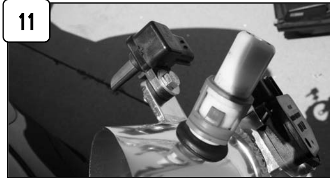
Install VSV valve to bracket on tube and secure using screw, flat washer, wavy washer and nut. Tighten using 10mm socket and wrench. Attach plastic fitting from step 4 to grommet on tube.
