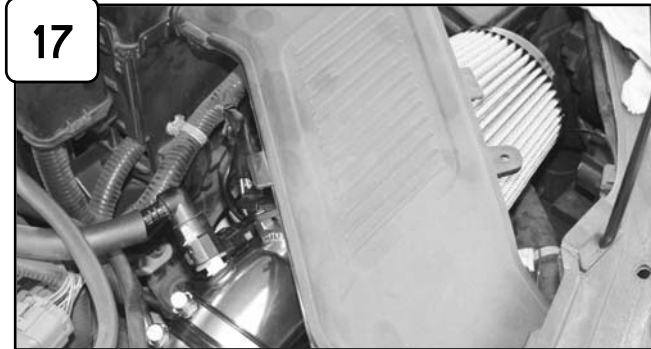
Install plastic battery ram air.
