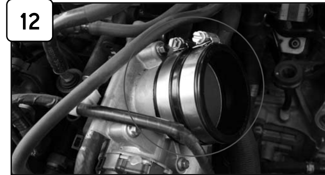
Attach coupling with clamps provided to throttle body. Do not tighten.
